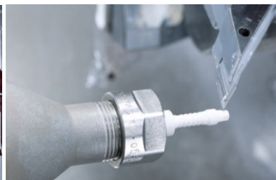
Lathe-turning a tooth implant
